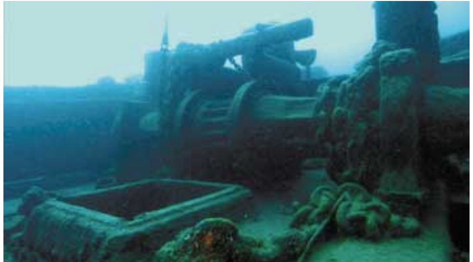
Figure 1: The windlass, an apparatus for winding in the anchor chain, stands virtually intact on the deck of E. B. Allen. Lying at a depth of 100–110 ft., the Allen and its cargo of grain were lost in a collision with the bark Newsboy off Thunder Bay Island on November 18, 1871. (All photos courtesy of Thunder Bay National Marine Sanctuary and Underwater Preserve).
