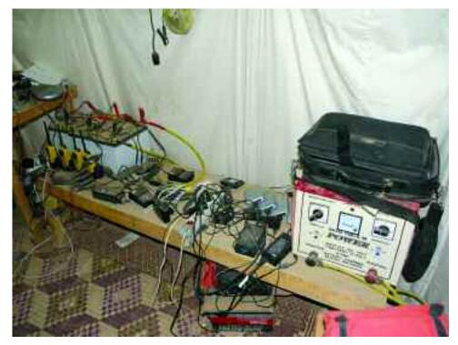
Figure 2. Power station for the ASPS project (Abydos, Egypt). To the right is a 12v battery charger that can be configured to charge up to five car batteries. To the left are a set of car batteries wired in parallel. A power inverter (the circular object in the upper left) is used to generate 22ov for the power strips seen in the photo. The remaining items (IPaq computers, walkie-talkies, and rechargeable AA batteries) are charged directly from 12V.
